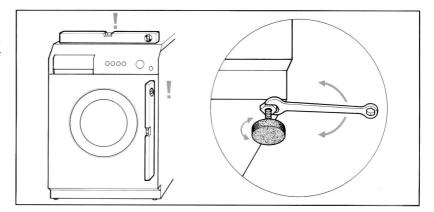
3.On appliances with **adjustable rear feet**, note that the rear of the appliance rests on skids and not on the feet. Before inserting the appliance into its place between the kitchen units, check that the rear feet are screwed fully in to prevent damage as the appliance is shifted into position.
